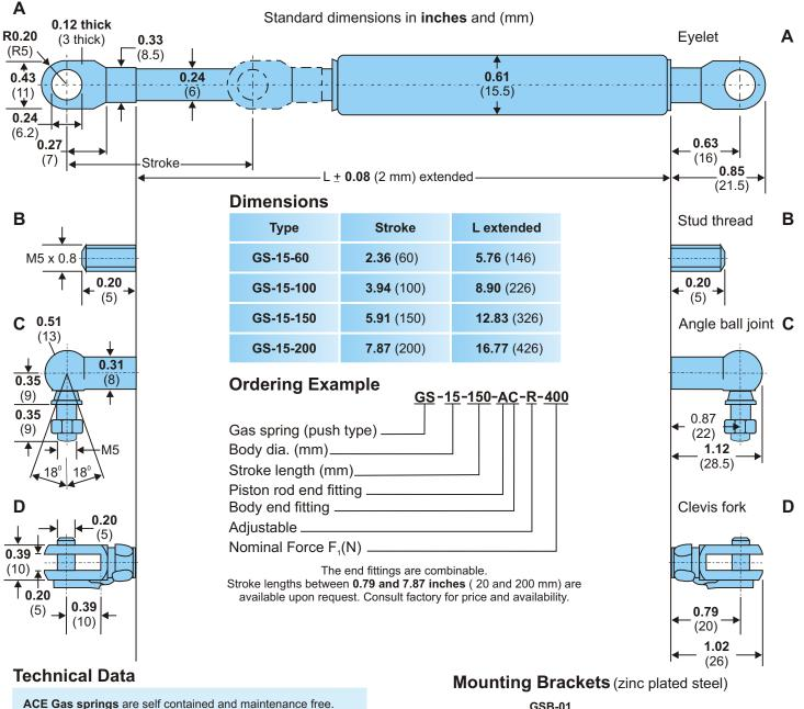
**Mounting position:** Can be mounted in any position, but we recommend mounting with piston rod downwards so that damping is effective at end of extension stroke.
